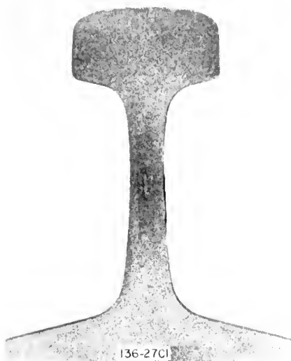
Fig. 15 (west rail)—Sound steel.
